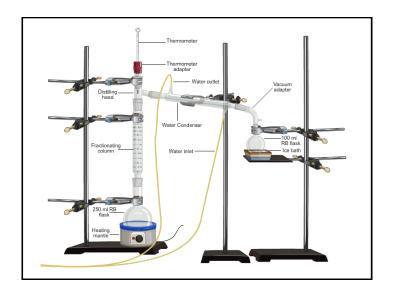
❖Vacuum distillation is a method of distillation whereby the pressure above the liquid mixture to be distilled is reduced to less than its vapor pressure (usually less than atmospheric pressure) causing evaporation of the most volatile liquid(s) (those with the lowest boiling points).
